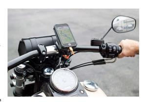
But high-power or high-volume motorcycle engines generate "intense high-amplitude vibrations", the support page says, which can be transmitted through the frame and handlebars. "Direct exposure to high-amplitude vibrations within certain frequency ranges may degrade the performance of these systems and lead to reduced image quality for photos and videos," it says. The solution is to refrain from attaching iPhones to the bike in the first place - something commonly done for navigation.
